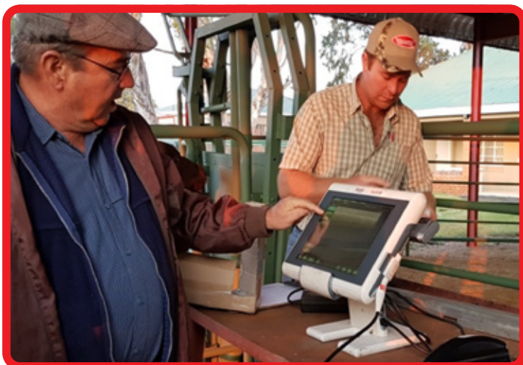
RTU Scanning apparatus comprises a probe and a screen to portray the RTU image.
